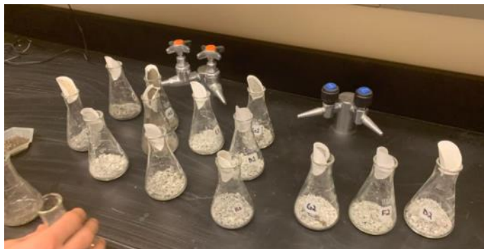
Figure 2: The sample flasks with each lithology composition. The filters from the post-leaching vacuum filtration are folded on top to analyze the loss of fine particles in the initial leach before the cycles begin.
