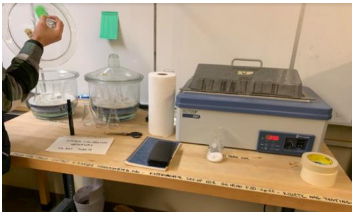
Figure 3: Desiccation chambers are on the left with flasks placed inside. The IsoTemp 220 water bath is set up on the right.
